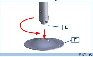
4º Insert the plug pin (E) in the hole on the ground fastening plate (F) and turn it 90° to fasten the plug to the plate.
