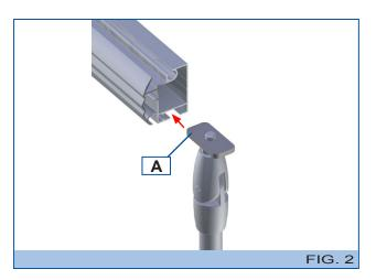
2º Insert the slide plate (A) in the end of the installed awning. After determining the permanent position for the pole, fasten the slide.
