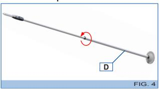
3. Holding the bottom part (D) still, turn the pole counterclockwise to lengthen and clockwise to fasten the pole in the desired position.
