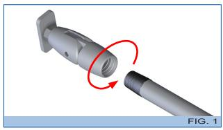
1º Fasten the pole to the joint by turning it counterclockwise, as shown in Figure 1.
